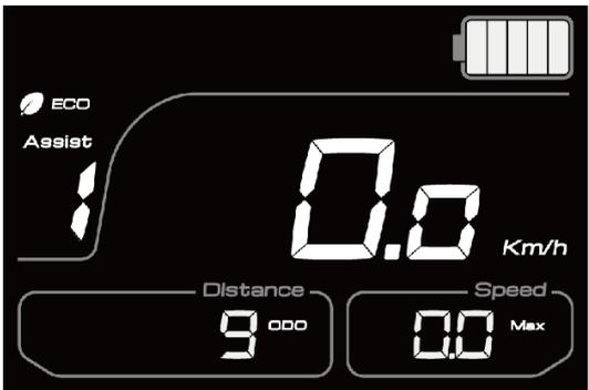
Figure4 - Normal indication interface after power-on
